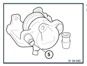
Check guide sleeves (5), fitting repair-kit guide sleeve if necessary.
