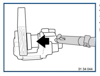
Carefully force piston out through connection bore with compressed air.
