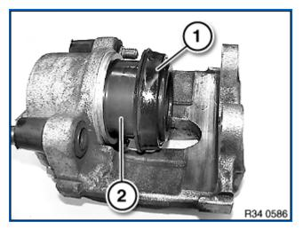
caliper housing must be kept dry. It must not come into contact with Ate brake cylinder paste or brake fluid so as to ensure that the dust sleeve is perfectly seated.
