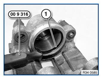
Carefully remove sealing ring (1) special tool 00 9 316.
