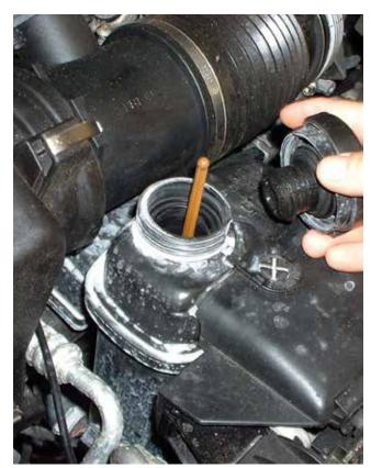
Just looking at the coolant in the overflow reservoir won't tell you much. You'll get a better idea of the level and corrosion situation by removing the radiator cap (engine cold, of course). The floating stick is a nice touch.
